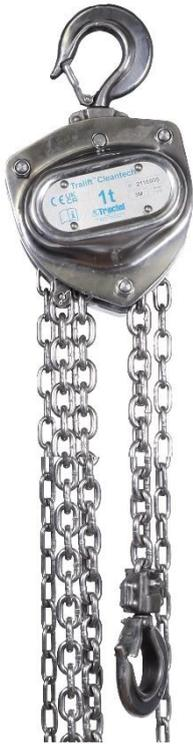
The Tralift™ Cleantech is a stainless steel chain hoist. It allows to lift and lower a load fixed to the lifting hook by means of human force applied to the hand chain. The device is anchored to a fixed attachment point or an interface (ex: Corso trolley)\* with the suspension hook.
